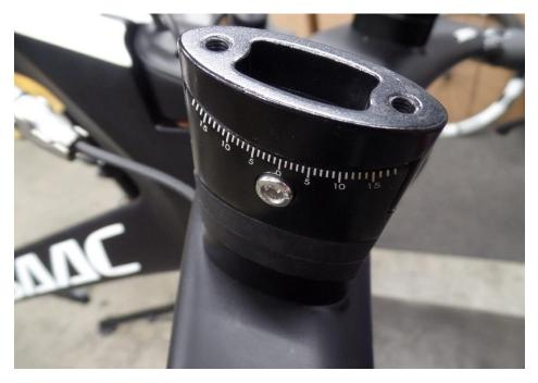
At last the carrier from the extensions should be mount on the alloy part.
