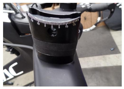
Inside of this top part the bolts should be mount, take care off the right length of this bolts. The bolts will fixed in the holes from the first alloy part:
