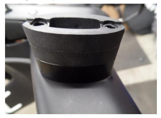
On the top of the plastic spacers the alloy part with the degreases should be mount:
